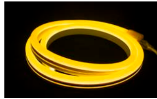
Amber LEDs Opaque Yellow Jacket (120V) 590nm • 21Lm/ft P2-NF-AY (120V)
