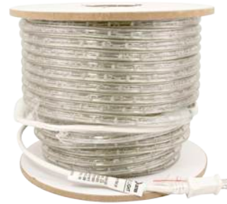
150ft Reel • 3/8" 120V Incandescent Rope Light MRL-CL-150 Clear, 5.5W/ft, 7.5Lm/ft MRL-AM-150 Amber, 5.5W/ft MRL-BL-150 Blue, 5.5W/ft MRL-PI-150 Pink, 5.5W/ft MRL-PU-150 Purple, 5.5W/ft MRL-YE-150 Yellow, 5.5W/ft
